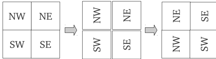
Figure 5.9: Rotation of a bitmap. Firstly, each piece is rotated individually. Then, a global rotation of the four pieces is done.
