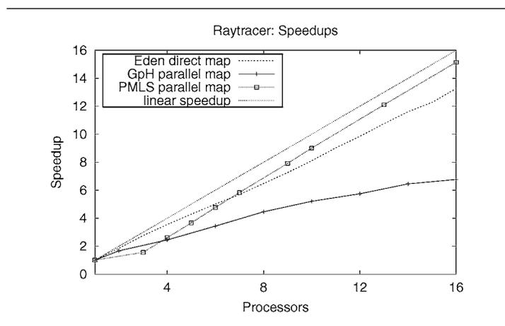
Figure 32. Speedups for raytracer on the Beowulf.
